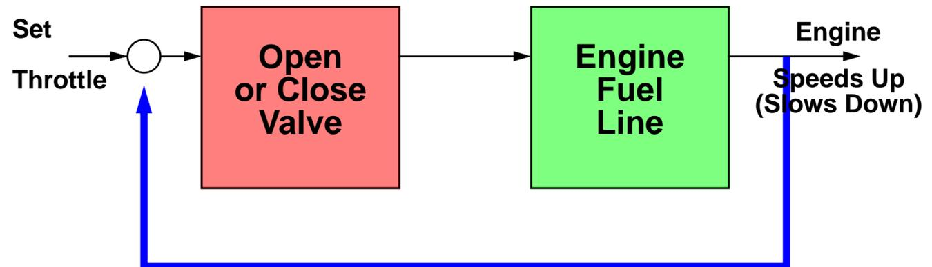
**Feedback: Engine shaft rotation speed**
