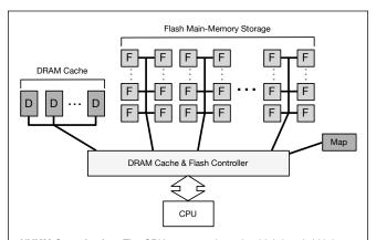
NVMM Organization. The CPU connects through a high-bandwidth interface to the NVMM hybrid DRAM/flash controller—this device controls both a large, last-level cache made from DRAM, and the flash subsystem. The NVMM controller maintains the flash mapping information in a dedicated DRAM while operating. When the system is powered down, the mapping information is stored into a dedicated flash location.
