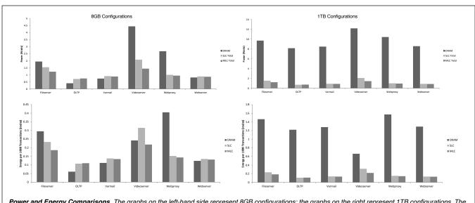
**Power and Energy Comparisons.** The graphs on the left-hand side represent 8GB configurations; the graphs on the right represent 1TB configurations. The graphs on the top present the average power consumed; the graphs on the bottom represent the energy per 1000 transactions.
