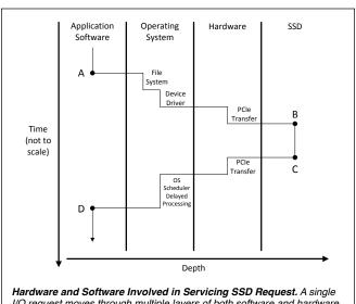
I/O request moves through multiple layers of both software and hardware.
