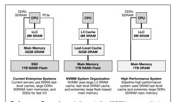
Performance Comparisons. In these studies, NVMM is compared to two different baselines. The first is the typical design practice today: using DRAM as main memory and SSDs as I/O. The second is the upper bound on achievable performance, simply extending current practice to use a DRAM main memory with as much capacity as in the SSD approach.
