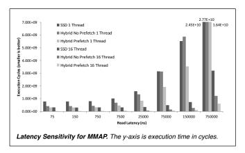
For the single threaded version of MMAP, the Hybrid architecture has roughly the same performance as the SSD for an MLC backing store. Turning on prefetching for the single threaded case does provide a boost of 1.6x. However, switching to the multithreaded case results in a large increase in per-
