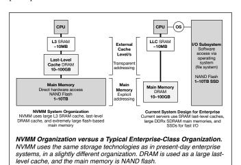
This paper introduces Non-Volatile Main Memory (NVMM), pictured above. NVMM is a new main-memory architecture for large-scale computing systems, one that is specifically designed to address the weaknesses described previously. In particular, it provides the following features:
