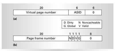
Figure 2. MIPS R2000/3000 TLB entry format: EntryHi (a) and EntryLo (b).
