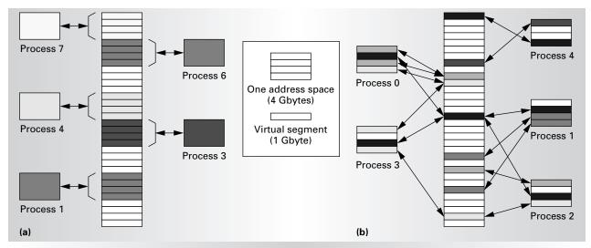
Figure 6. Difference between ASIDs and segmentation in two virtual addressing schemes. A 3-bit ASID extends the 32-bit address space (a). A 35-bit segmented address space is divided into fixed-length, 1-Gbyte segments (b). In both schemes, processes generate 32-bit virtual addresses, and the hardware translates a 35-bit virtual address.
