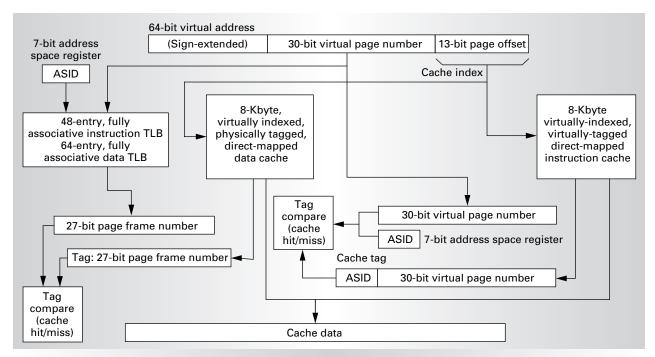
Figure 4. Alpha 21164 address translation mechanism. The virtual bits of the page offset effectively physically index each of the 8-Kbyte split caches. The data cache is physically tagged and the instruction cache is virtually tagged. The instruction TLB is accessed every reference to provide page protection.
