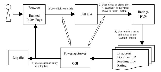
Figure 3. Procedures for using the modified Powerize Server 1.0
