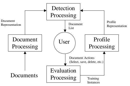
Figure 1. Content-based filtering system model
